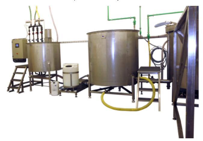
New Back flush system provide cleaner and higher quality Brine mixture.
