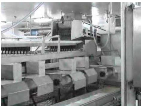
Easy grader with 20 grading lines and 5 grading conveyors
