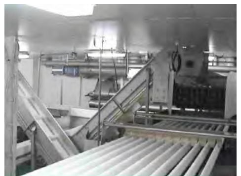
Easy grader with 3 grading lines and 4 grading slots
