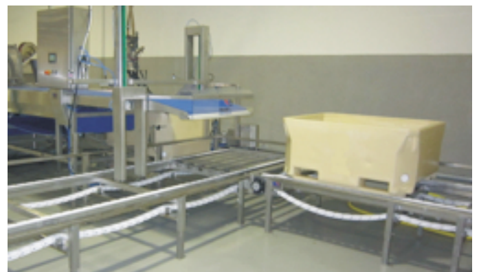
TR 850 injector, Easy Layer & Automatic Tub System
