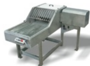
Easy Flaker that flakes frozen minced fish block for Easy-Inject. "Fish in Fish"
