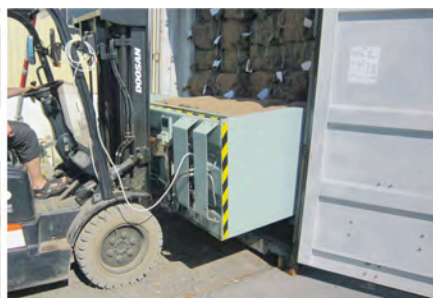
Loading container with Easy Container Stacker
