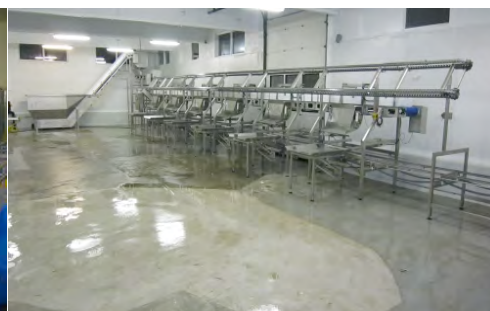
Fillet-line with 6 work stations
