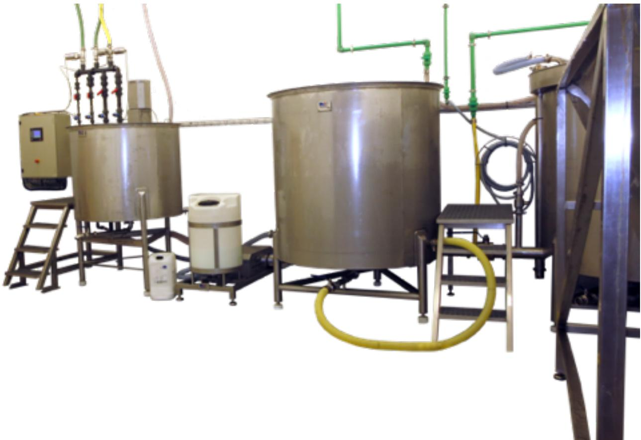
New Back flush system provide cleaner and higher quality Brine mixture.
