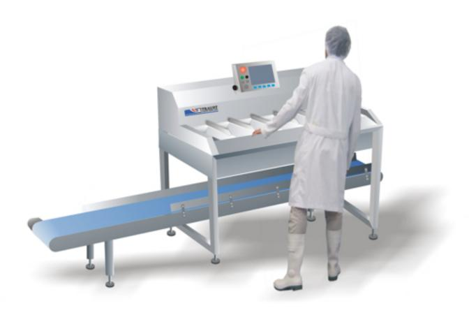
The Easy Weight Batcher is a unique weighing machine that combines a predetermined number of fresh or frozen products into a package with an exact weight.
